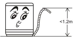
Confirm the end of drain hose is higher than the level of tub. If not the siphon will being.
